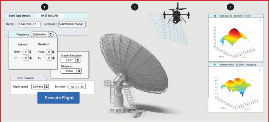
▲ Fig. 1 Raster scan process diagram.
